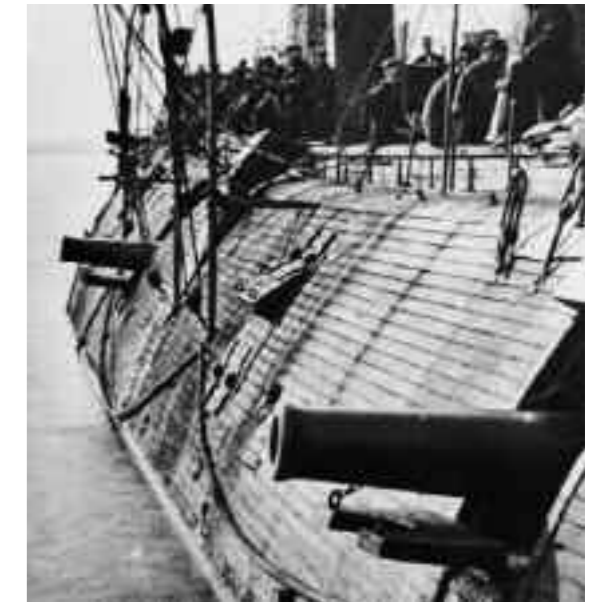
ABOVE: Launched February 14, 1862, the screw-steamer USS Galena (actually an ironclad) once competed for navy contracts with the USS Monitor . She carried eight 9-inch Dahlgren smoothbores, two of which can be seen protruding from her ports.
